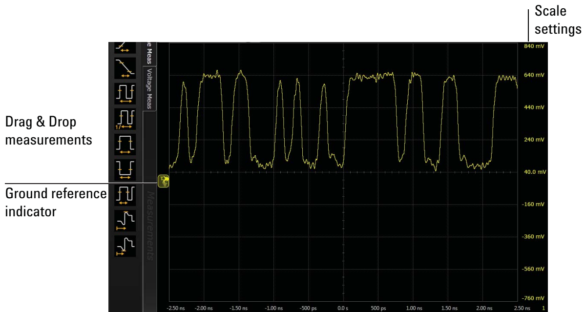
Figure 13 Infiniium oscilloscope waveform display area
